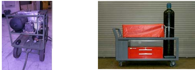
Figure 6-14. Green and Red Nitrogen Charge Carts (available at test sites)
